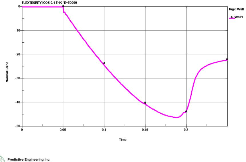
All Results Confidential and Proprietary George.Laird@PredictiveEngineering.com 1.800.345.4671 The peak load carrying capacity is around 46 lbf. After this load the structure buckles or collapses and the load decreases.
